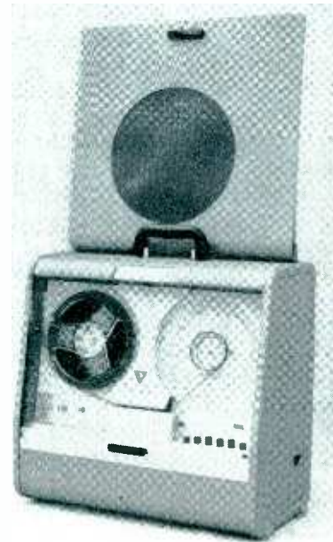
Top: the recorder shown closed, both front and back. The front drops down like a roll top desk. The shape of the recorder makes it very convenient for carrying. The lower illustrations show how the back panel, carrying the ten-inch speaker is swung up into playing position. It may also be operated with the case closed. Phonograph type locking arms hold the speaker in position. The microphone attaches to a small bracket.
