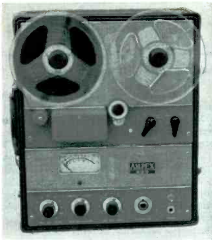
The 600 may be used either vertically or horizontally. Reels are held in place by rubber knobs which grip the drive shafts.
