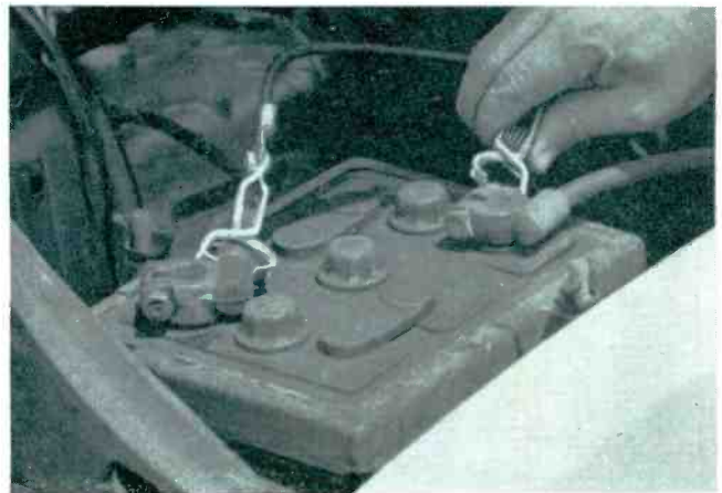
to the engine block instead of the battery. Be sure to attach the "ground" lead to the proper battery terminal.
